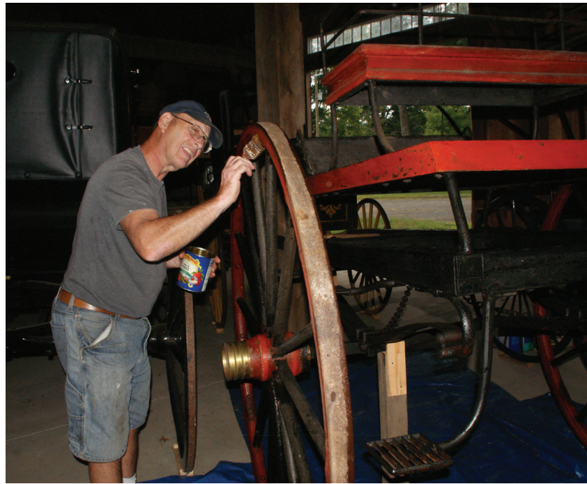
Jim Kent applies linseed oil to the rim of a giant wheel on the King House Museum's old hunting trap, once owned by Hugh Swinton Legare of Kent Place.
